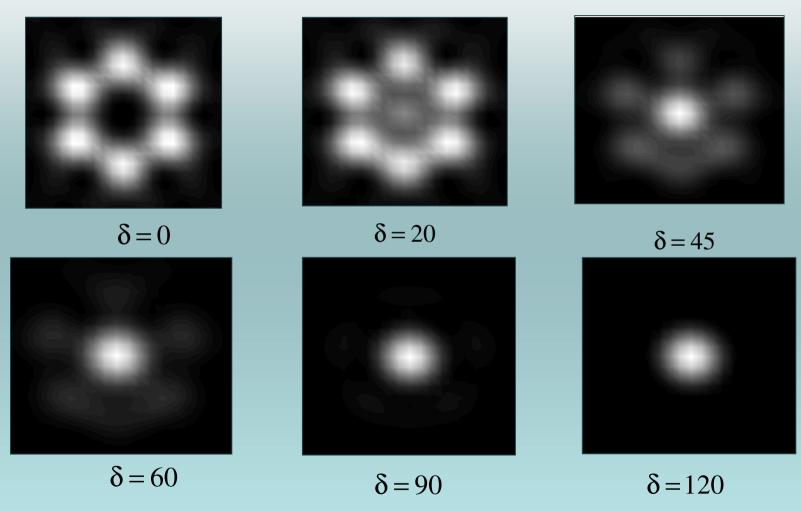
Three-films interference coatings may to vary the phase shift upon reflection and control the angular width of the pattern and its form.
