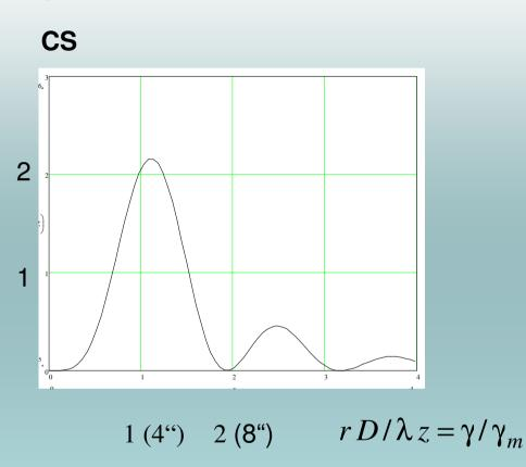
Another way to optimize the pattern is to make a gradient surface on the CCR front face. Instead of the Airy diffraction pattern, several rings are observed; the brightest ring is at an almost optimal angular distance for the GLONASS system.
